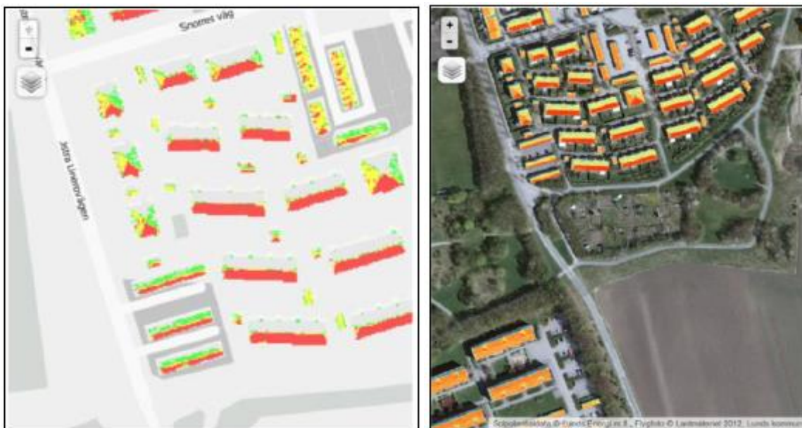
Two different display views for Solkartan. The colors indicate whether the amount of sunlight hitting each roof is Very good (red), Good (yellow) Less good (green) or Not suitable (gray).
